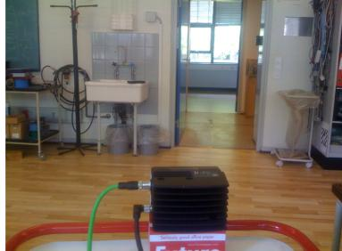
The integration time is set to 200/2000, this is the highest integration time that can be supported with the power supply used. One image is taken with each modulation frequency, and one image is taken with dual modulation frequencies.
