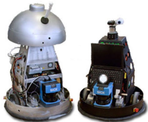
Figure 12: Two of the larger mobile robots from the AUT department of DTU
