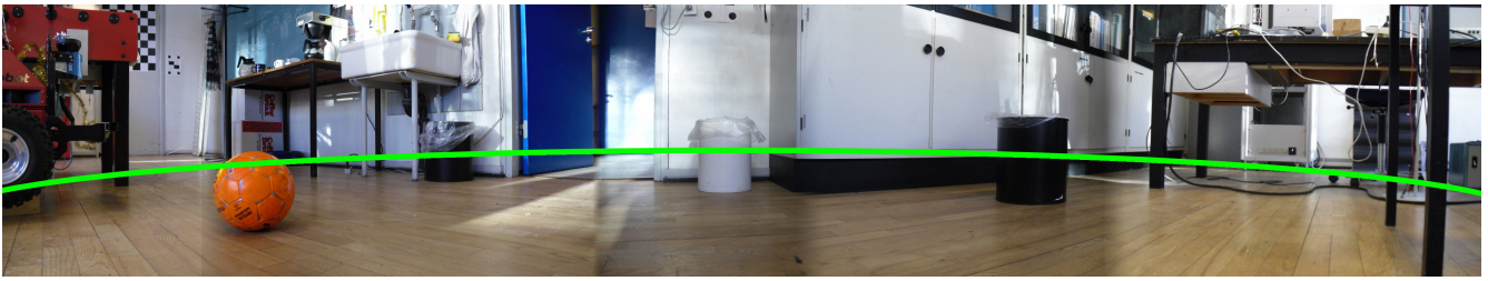
Figure 3: Merge of 5 pictures taken from the same origin. Green overlay is approximate laser-scan.
