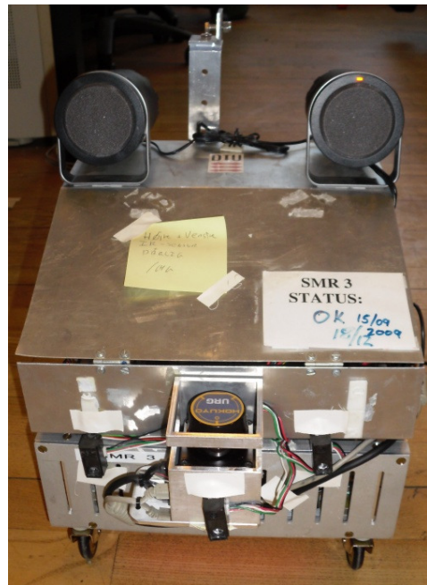
Figure 7: Small Mobile Robot (SMR) with repositioned laser scanner.
