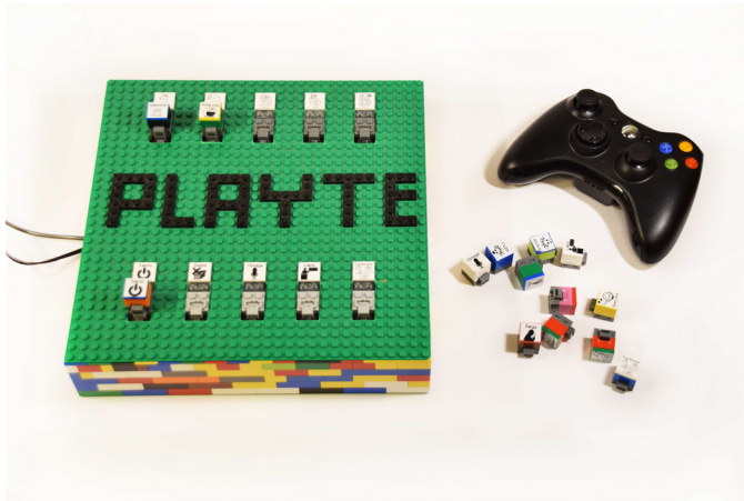
Fig. 2. The Playte is a tangible interface for easy accessible behaviors-based robot control. Shown are also preprogrammed behavior-bricks and trainable bricks, as well as a gamepad used for training/recording new behaviors and for direct remote control.
